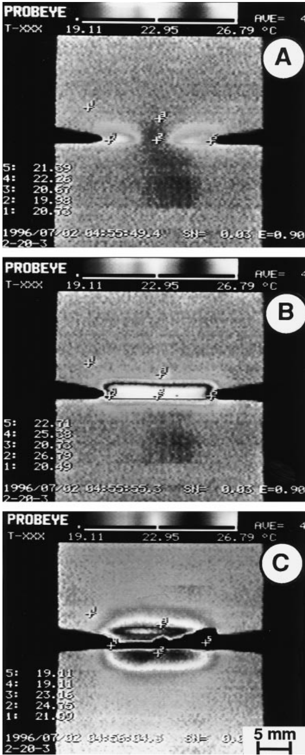
Fig. 6. Serial IRT frames taken during loading of a DDEN-T specimen of l \approx 20 mm of PEN-2 Note: the taking position of the IRT frames are shown in the related F-x curve in Fig. 5.
